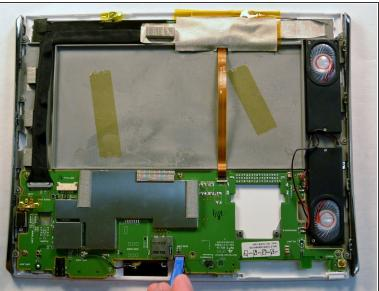
Remove the zero insertion force connector (ZIF) by using a plastic opening tool, spudger, or fingernail to lift retaining flap.
