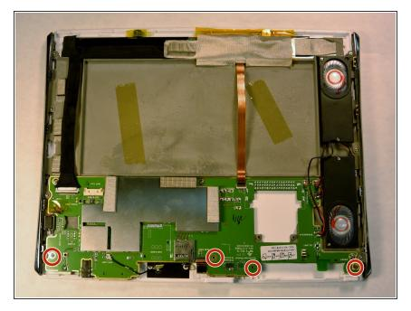
Remove the four 3.5 mm Phillips #00 screws from the circuit board near the bottom of the tablet.
