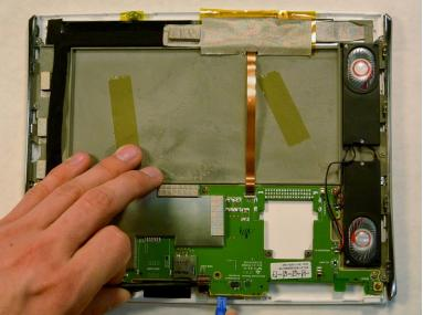
Slightly lift up the green electrical board and pull out the camera.
