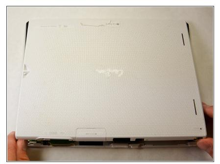
Once the front and back faces are completely separated, remove the back cover to reveal the inside components.
