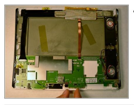
Pull out the volume rocker by carefully moving it side to side with your fingers.
