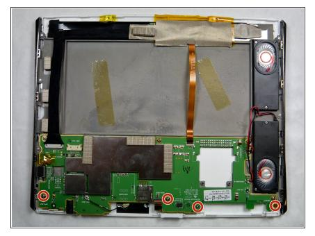
Remove the four 2.5 mm Phillips #00 head screws from the circuit board near the top of the tablet.
