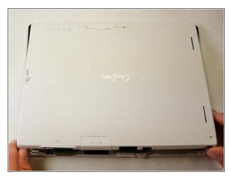
Once the front and back faces are completely separated, remove the back cover to reveal the inside components.
