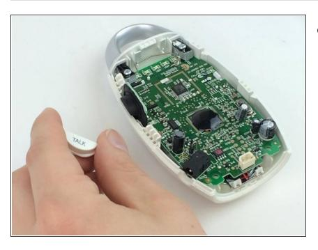
Remove the "TALK" button to get access to remove the motherboard.
