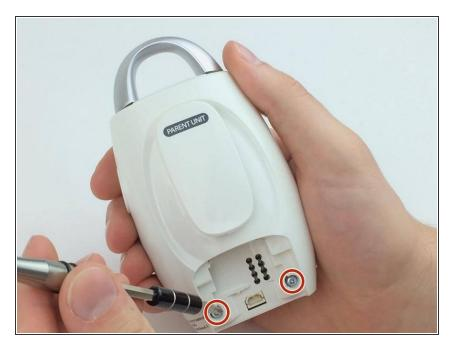
Using the Phillips #00 screwdriver, unscrew the two 5.0 mm Phillips #00 screws at the bottom of the monitor.
