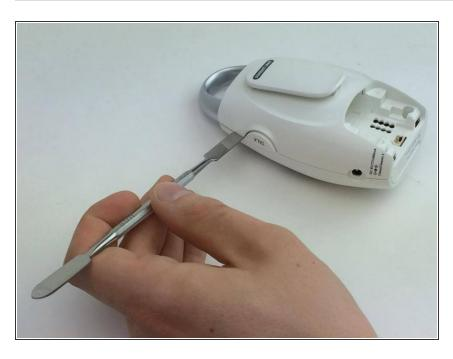
Separate the back half of the device from the front using the metal spudger.
