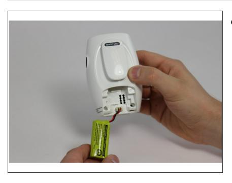
Unplug the battery from its connector and remove.
