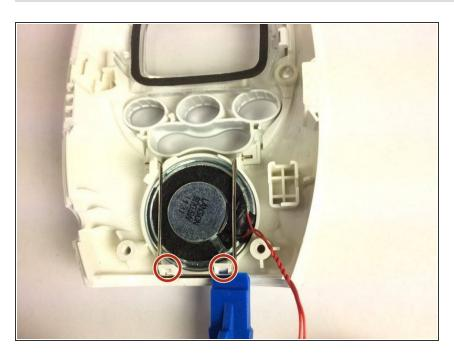
Use the plastic spudger to push the two white plastic tabs, at the bottom of the device, up to release the metal retaining clip.
