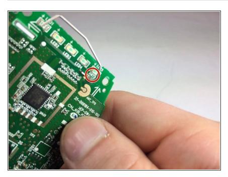
Push down on the antenna, located on the top of the motherboard.
