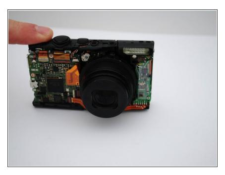
Manually remove the front panel from the camera.
