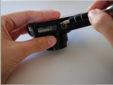
• Unscrew the two 4 mm Phillips head screws from the bottom side of the camera.
