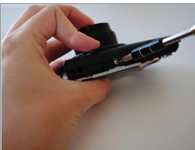
Unscrew the one 3 mm Phillips head screw on the top of the camera.
