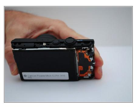
The back side of the camera should pop off or be removed by hand.
