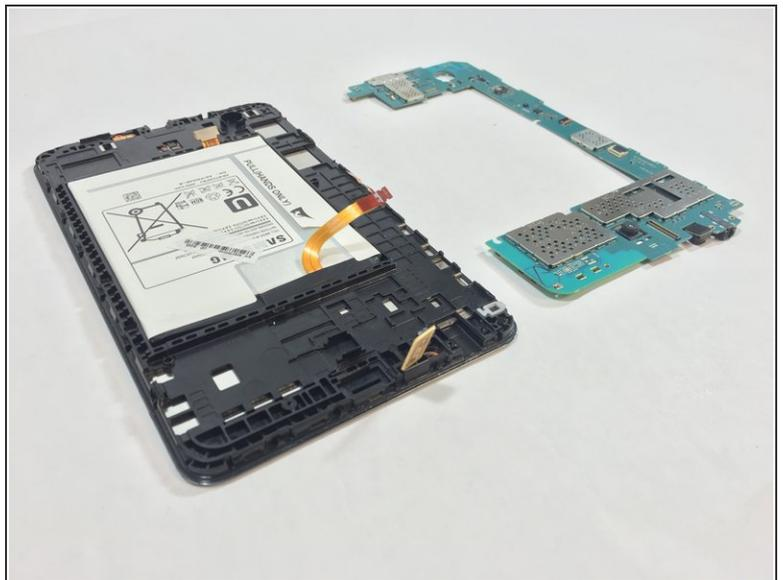
⚠ Use extreme care while removing the motherboard to avoid damaging the component.
