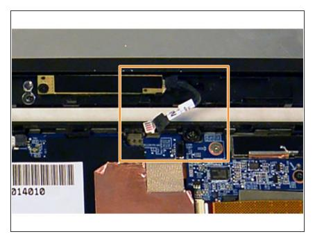
Disconnect the camera cable from the device backing.
