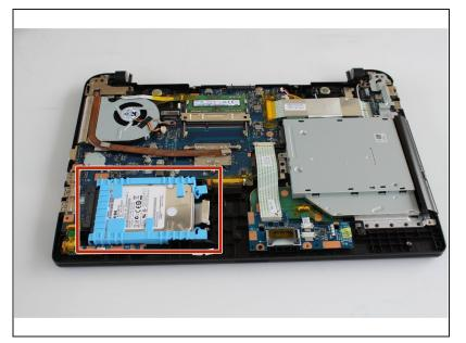
Once the device is open from the bottom, look for the bright blue plastic frame which encases the hard drive
