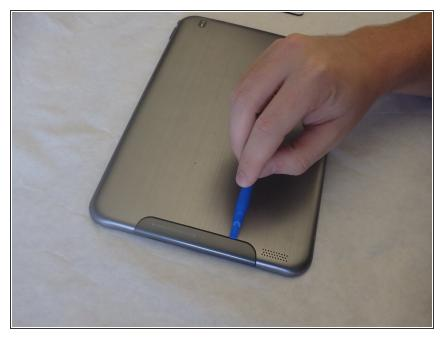
Remove the cover over the Micro SD outlet by using a plastic opening tool to pry open and push out the cover panel.
