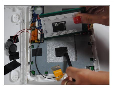
Use a spudger to separate the battery from its adhesive.
