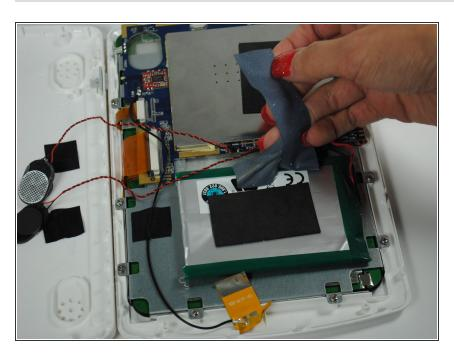
Remove the black tape holding the battery in place.
