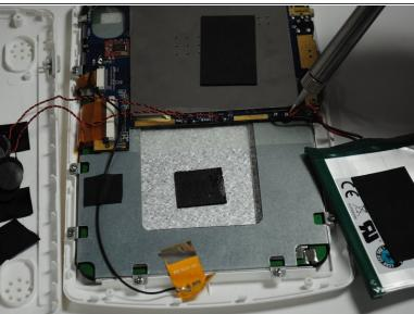
Use a soldering station to separate the battery from its connecting wires.
