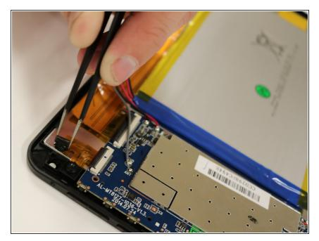
Insert the tweezers into the black part of the ZIF connector and lift it in an upwards motion. By lifting the connection, you will see it will free the circuit strip.
