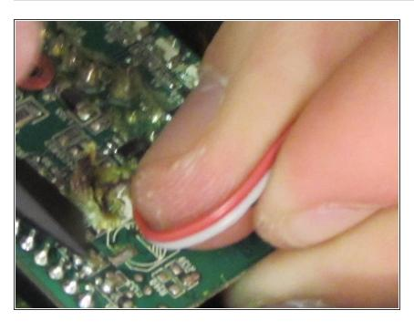
Once you have soldered the glue off, remove the wires by pulling upwards. To reassemble your device, follow these instructions in reverse order.
