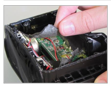
Remove the foam padding located in the Braven BRV-1s.
