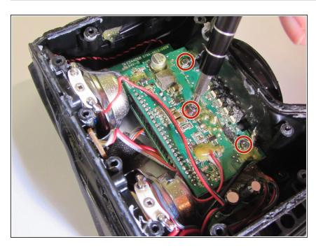
Using a 0mm Philips Head screwdriver unscrew the three 0.6mm screws on the auxiliary circuit board.
