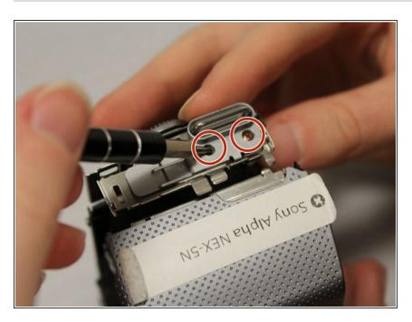
Unscrew 2 copper 1.2 mm Phillips #000 screws underneath the lanyard loop (near the control wheel).
