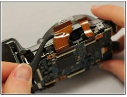
Locate 3 thick ribbon cables on the bottom, and flip up the white retaining tabs. Pull out the remaining ribbon cables, utilizing tweezers.
