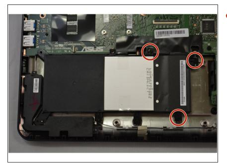
Remove the three 5mm Phillips #0 screws securing the battery.
