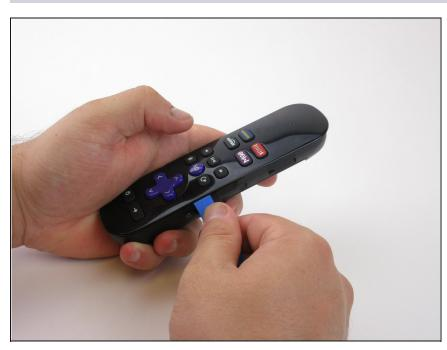
Use a plastic opening tool to pry open the remote.
