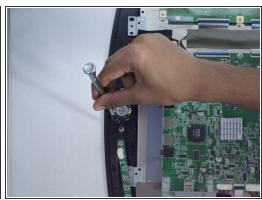
• With the Phillips #01 screwdriver, remove the four 5 mm length x 7 mm head screws from the assembly (two for each side speaker).
