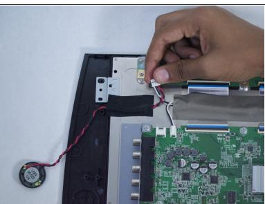
Remove the speaker by depressing the white tab on the speaker wire connector.
