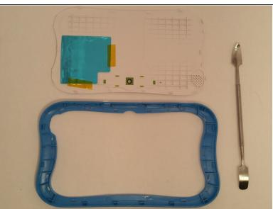
There are 19 tabs that need to be pushed out of the inner trim. The metal spudger works great here.
