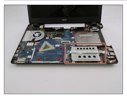
Locate the hard drive in the metal casing.
