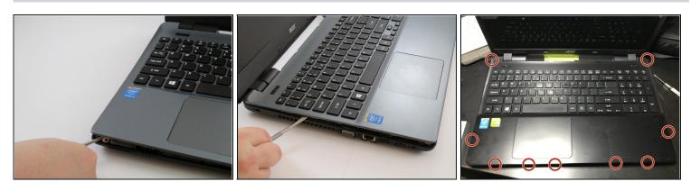
• Carefully pry apart the clips holding the keyboard in place by moving a metal spudger along the seam.
