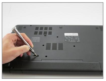
Place the pointed end of a spudger into the battery lock.
