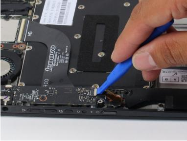
Using the plastic opening tool, flip open tab as shown.
