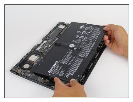
Carefully lift and remove the battery.
