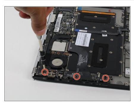
Remove the three indicated 3.5 mm screws using the Philips 00 screwdriver.
