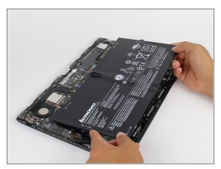
• Carefully lift and remove the battery.
