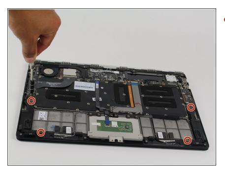
Remove the four 4 mm screws using the Phillips 00 screwdriver.
