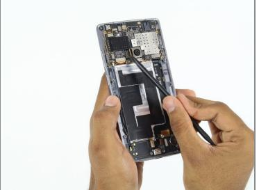
Use the spudger tool to pry off the connection on the left of the front facing camera.
