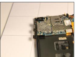
Using a pry tool, gently lift the side control buttons assembly away from the case. They should be loosely connected to the motherboard.
