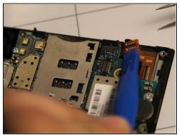
Separate a cable ribbon from the top right of the motherboard - near the cable from the previous step - by gently inserting the pry tool under the rectangular metallic piece and lifting.
