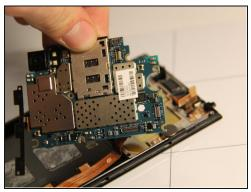
• Remove the motherboard from the panel carefully. Use the pry tool as a lever from the top of the panel and lift if from that side.
