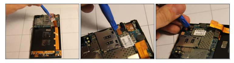
• Separate a cable ribbon from the top right of the motherboard by gently inserting the pry tool under the rectangular metallic piece and lifting.
