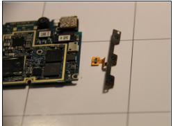
• With the motherboard removed flip it over onto its front and use a small pry tool to gently disconnect the side buttons from the back of the motherboard.
