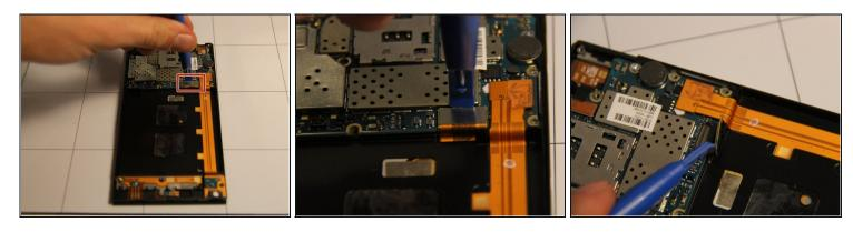
• Use a pry tool to separate the LCD display cable from the motherboard. The cable connects to the motherboard as a rectangular metallic piece at the bottom right of the motherboard.
