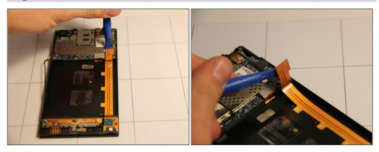
• Disconnect the gold ribbon cable for the LCD display by gently inserting the pry tool under the wide end and lifting up.
