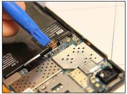
Using a spudger, remove the small ribbon cable that is connected to the battery.
