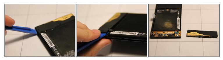
• Remove the plastic cover on the bottom of the back panel by inserting the pry tool at the edge and gently lifting.
