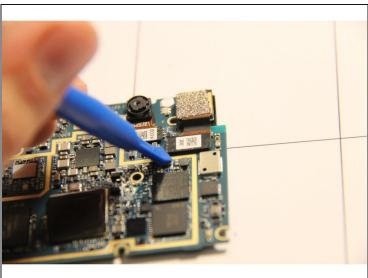
• After removing the motherboard, use a pry tool to gently remove the camera's ribbon cable from the motherboard.
