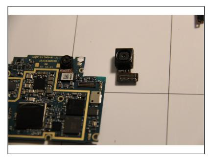
The rear facing camera is now removed from the panel successfully.
