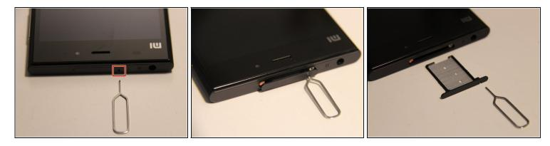
• Firmly press the SIM card removal tool into the hole located at the top of the phone to eject the SIM card tray from the slot.
