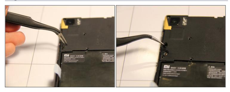
• Using tweezers, remove the rubber dust cover on the back panel of the phone.
