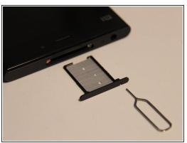
Firmly press the SIM card removal tool into the hole located at the top of the phone to eject the SIM card tray from the slot.
