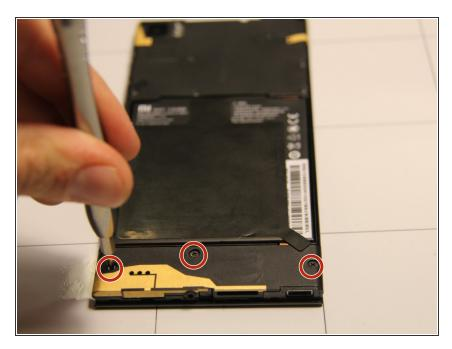
Next, remove these three screws located at the bottom of the back panel.
