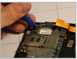
Separate a cable ribbon from the top right of the motherboard by gently inserting the pry tool under the rectangular metallic piece and lifting.
