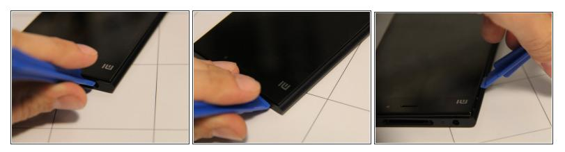
Insert a pry tool into the upper edge of the phone, where there is a small gap between screen and frame of the phone to begin separating the screen from the rest of the phone.
