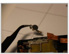
With the motherboard removed you can use tweezers to remove the vibrator rather easily.
