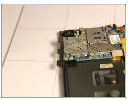
Using a pry tool, gently lift the side control buttons assembly away from the case. They should be loosely connected to the motherboard.
