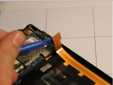
Disconnect the gold ribbon cable for the LCD display by gently inserting the pry tool under the wide end and lifting up.
