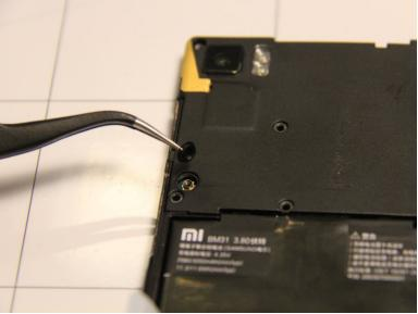
• Using tweezers, remove the rubber dust cover on the back panel of the phone.
