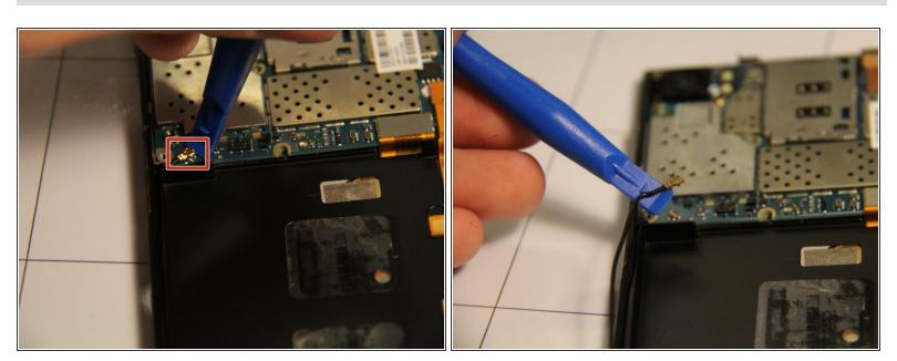
Disconnect the antenna wire that is attached to the lower left side of the motherboard using the pry tool.
