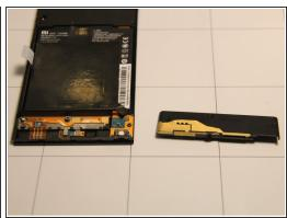
Remove the plastic cover on the bottom of the back panel by inserting the pry tool at the edge and gently lifting.
