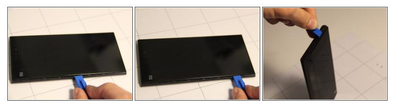
• Once the pry tool has been inserted into the phone, slide it around the perimeter of the phone while gently lifting until the screen panel and back panel of the phone separate.
