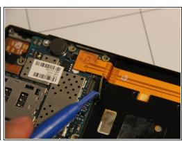
• Use a pry tool to separate the LCD display cable from the motherboard. The cable connects to the motherboard as a rectangular metallic piece at the bottom right of the motherboard.
