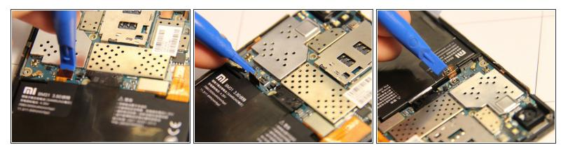
Using a spudger, remove the small ribbon cable that is connected to the battery.
