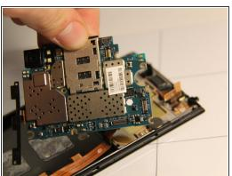
Remove the motherboard from the panel carefully. Use the pry tool as a lever from the top of the panel and lift if from that side.
