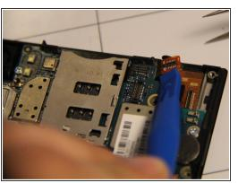
Separate a cable ribbon from the top right of the motherboard - near the cable from the previous step - by gently inserting the pry tool under the rectangular metallic piece and lifting.
