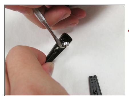
• Use a nylon or metal spudger set to lift out the microphone.
