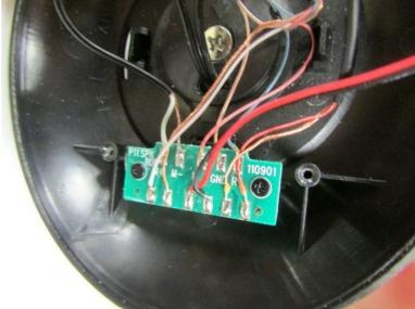
Inspect the wires for damage as illustrated
