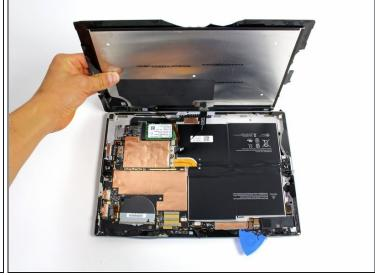
Lift the screen up carefully so that no wires are torn.
