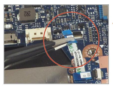
Use a pair of tweezers to disconnect the motherboard-side of the SD board ribbon cable. Gently lift up the black tab, and then ribbon cable should come free from the ZIF connector.
