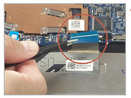
Use a pair of tweezers to disconnect the keyboard ribbon cable from the motherboard ZIF connector. Gently lift up the white tab, and the cable should come free.
