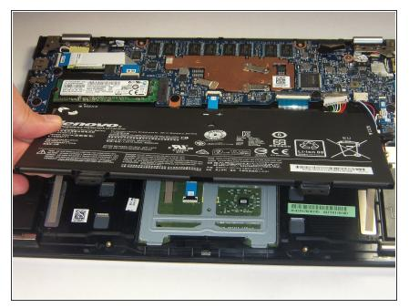
• Carefully remove the battery from the device.
