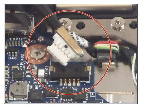
Use the tweezers to unplug the USB port from the motherboard by gently lifting the white connector up from the black motherboard connector.
