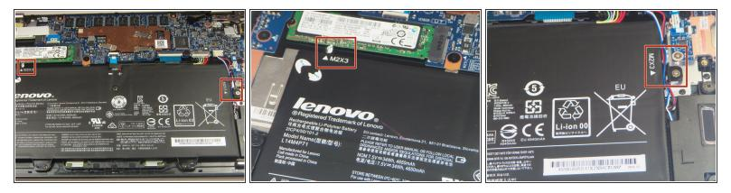
• Remove the two 3 mm Phillips #00 screws securing the battery.
