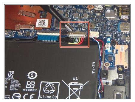
• Use a pair of tweezers to gently disconnect the battery connector.
