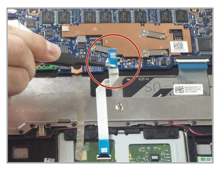
Use a pair of tweezers to disconnect the motherboard-size of the trackpad ribbon cable. Gently lift up
