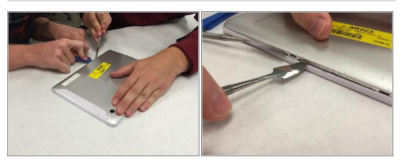
• Use a prying tool to pry the back panel from the tablet chassis. Pry the panel at different locations around the device to separate clips.
