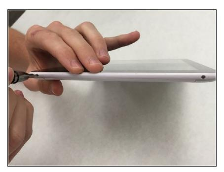
remove the screws at the four corners of the device.
