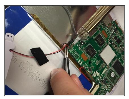
Use a soldering iron to remove power cables from battery. The power cable is shown at the corner of the battery in the picture.
