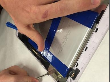
Use a tool to carefully pry battery away from chassis. The battery is attached by an adhesive.
