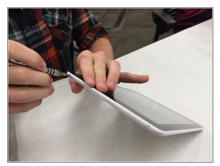
Use a Philips screwdriver to remove the four screws: two at the top and two at the bottom of the device.
