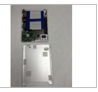
Place the device screen down on the table and use a pry tool to remove the back panel.
