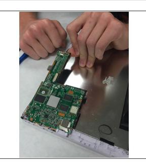
Remove the screw attaching the motherboard to the back panel. Gently remove the motherboard.
