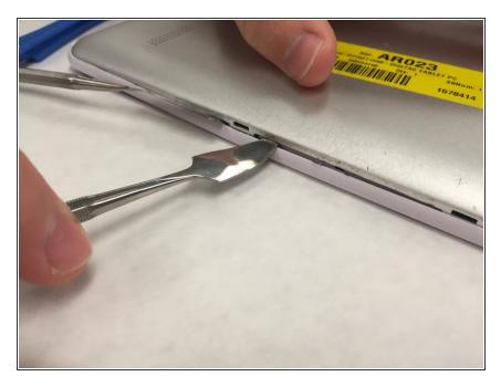
Remove the back panel of the device using an opening tool.
