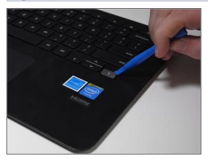
Use the plastic opening tool to loosen a key of choice.
