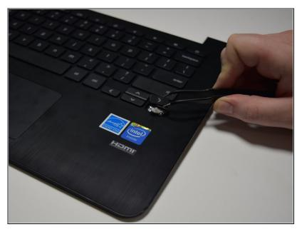
• Removed the loosened key with the <u>tweezers</u>.
