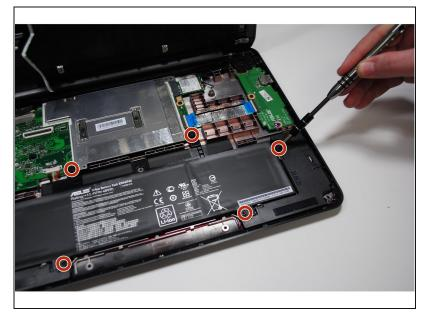
Remove the 6.0mm Philips screws from around the battery. Make sure to disconnect the battery from the motherboard.
