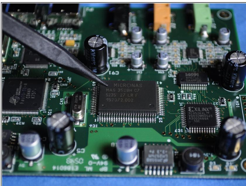
ⓘ Here we have the Micronas MAS 3529H Dolby Digital and Mpeg2 Layer 2 Audio Decoder. Its the heart of the sound card, without it, there would be no 5.1. Dolby labs made a contract with Micronas to manufacture these chips under specifications.
