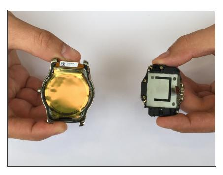
Carefully pinch out the battery case with your fingers to remove it from the face of the watch.
