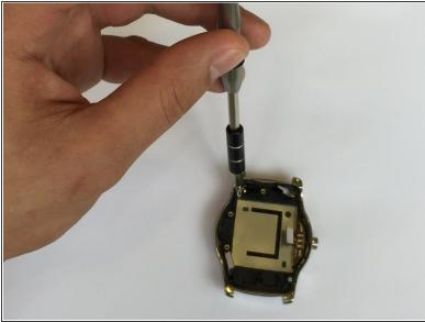
Use the PH000 screwdriver to remove the two highlighted screws to release the battery
