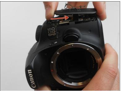
Using the plastic opening tool, carefully pry off the the side cover.
