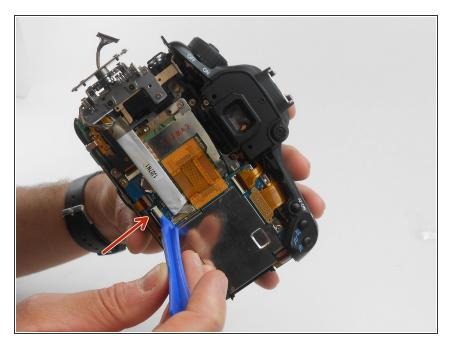
Carefully pry off the LCD screen connector up from the motherboard to disconnect it, using the plastic opening tool.
