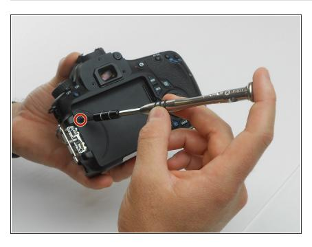
Using the PH00 screwdriver, remove the 3.8 mm Phillips #PH00 screw located on the back of the camera.
