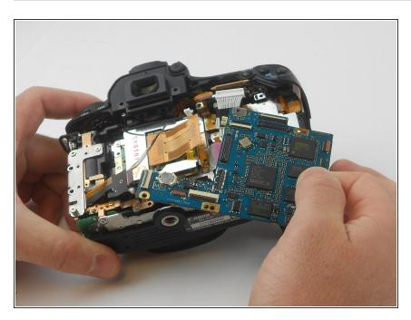
With every wire properly removed, the motherboard can now be lifted out of the camera.
