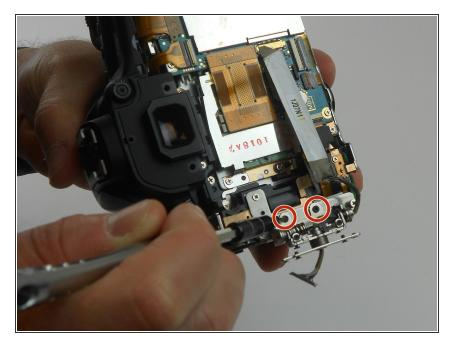
Remove the two 2.8 mm Phillips #PH00 black screws on the back of the swivel assembly using the PH00 screwdriver.
