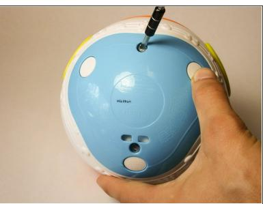
There are two screws that require a 4.0mm flat head screwdriver. Twist them counter clockwise to remove. When you remove them they stay contained within the blue outer case.
