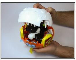
Remove 6 screws in order to pop off the outer shell and reach the inside components.
