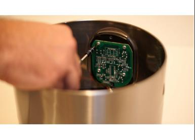
Using a Phillips head screwdriver, size PH2, remove the four screws holding the interface in place.
