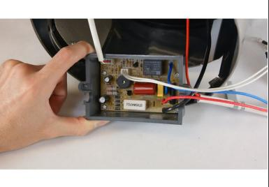
Using a Phillips head screwdriver, size PH2, remove screws from the control module to expose wired connections.
