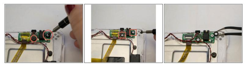
• Remove the two black 3.5 mm Phillips # 00 screws and the attached washers.
