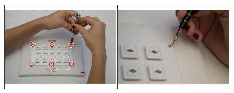
• Remove the six 2.5 mm JIS #000 screws attaching the custom grid to the back panel.
