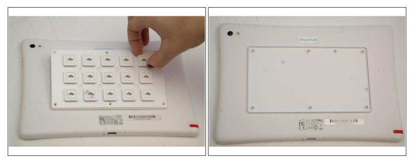
Grasp one of the protruding squares and gently lift off the back plate. Place it aside for later reassembly.
