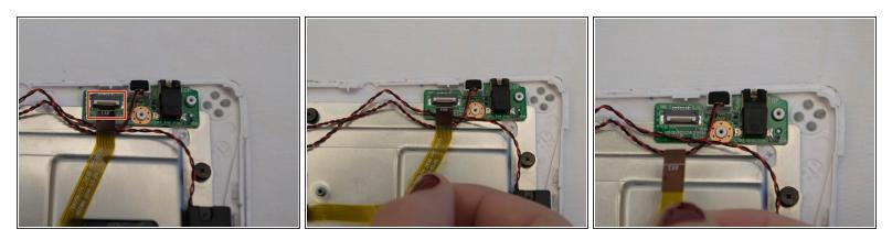
• Lift the white part of the connector and pull out the connector.
