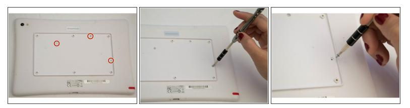
• Remove the three 3.5mm screws using the J-0 screwdriver attaching the back panel to the device.
