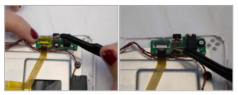
• Remove the yellow plastic tape from the connector with tweezers.
