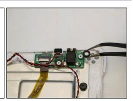
• Remove the two black 3.5 mm Phillips # 00 screws and the attached washers.
