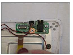
• Lift the white part of the connector and pull out the connector.
