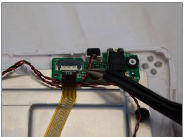
• Remove the yellow plastic tape from the connector with <u>tweezers</u>.
