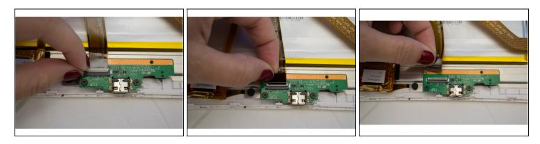
• Disengage the white lock keeping the plastic ribbon in place.
