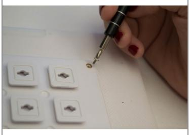
• Remove the six 2.5 mm JIS #000 screws attaching the custom grid to the back panel.
