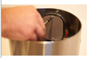
Remove the two screws holding the cardboard cover over the Interface using a Phillips head screwdriver, size PH2.
