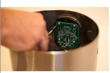
Using a Phillips head screwdriver, size PH2, remove the four screws holding the interface in place.
