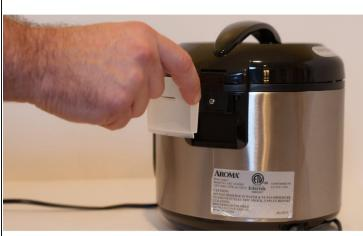
The first step is removing the condensation catcher in order to reach the control panel. We do
