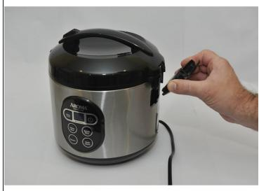
Gently remove the piece that was held in place by the screw, you do this by pulling out from the top, then pulling up. This will expose the hinges for the lid.
