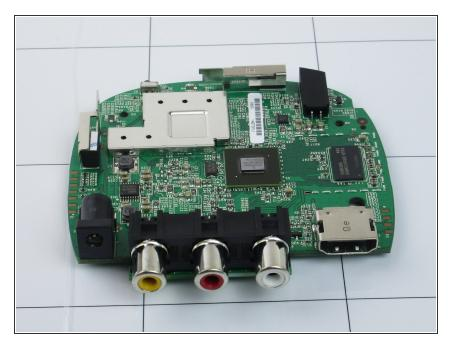
Remove the board from the plastic enclosure.
