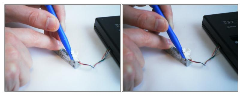
Remove the glue on the third side so that the wires are completely disconnected from the sensor.
