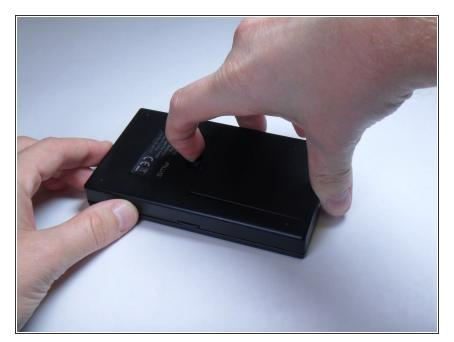
Flip the device over and remove the battery cover.
