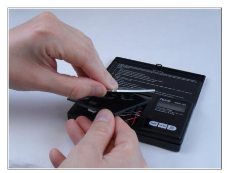
Using your hands or a plastic opening tool, peel back the metal plate from the plastic underneath.
