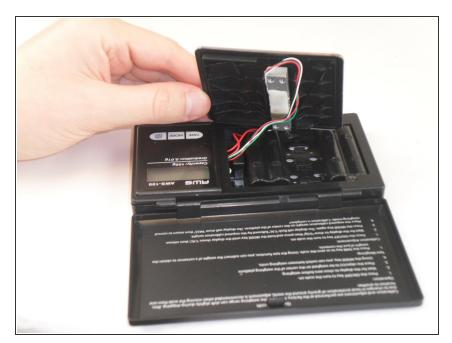
Once the screws are removed, lift up the metal weighing plate with your hands. At this point in the process, the sensor will still be attached.
