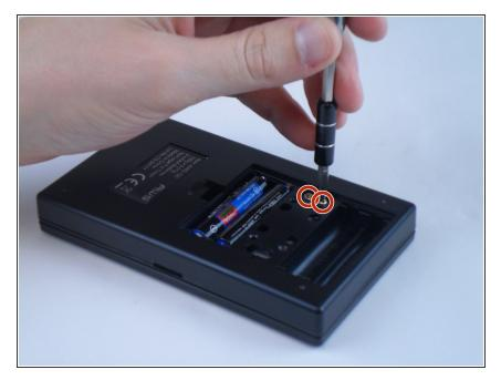
Remove the two screws (length: 7/16") located underneath the battery cover. Use a Phillip's head number 1 screwdriver.
