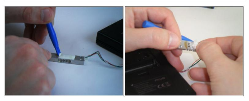
With the sensor detached, use a plastic opening tool to peel away the glue holding the wires.
