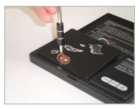
Using the same screwdriver as before, remove the two screws (length 3/8") on the plastic plate connected the sensor.
