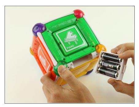
Gently pull out the battery cartridge and if needed, replace the batteries with 3 AA alkaline batteries.
