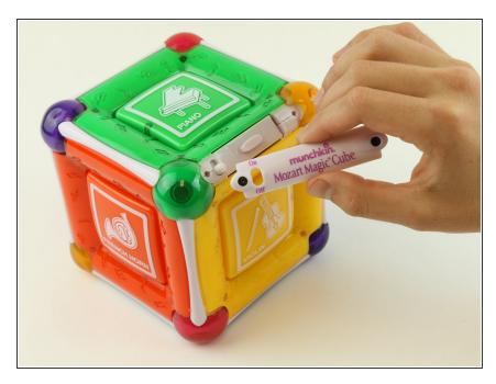
Remove the On/Off switch plate and save the screws so you can use them later to put the plate back on.
