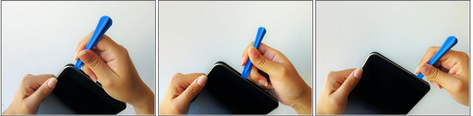
**⚠** Before disassembling your Samsung Galaxy Tab 4 8.0, be sure it is powered off and you remove the SIM and Micro SD cards.
