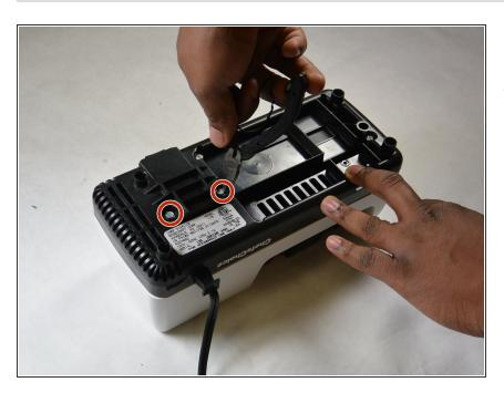
Remove the two hex-cap screws on the bottom using a pair of pliers.
