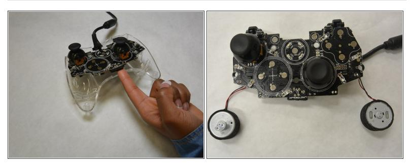
• Lift the Logic Board and remove the rumble motors from the base of the controller.
