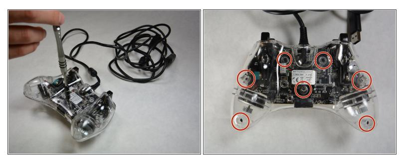
• Loosen the seven 11 mm Phillips #0 screws located on the back of the controller.
