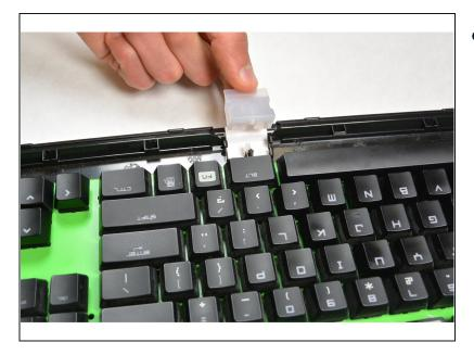
• Lift the covering of the LED logo vertically out of the slot.
