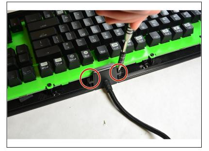
Find where the cable enters the back of the keyboard. There are two screws on either side of the tab holding the cable in. Once removed, the tab should slide out of the keyboard.
