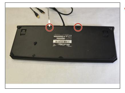
There are two tabs on both sides of where the cable enters the back of the keyboard. Use the metal spudgers to gently pull up the tabs. These are circled in red on the picture.
