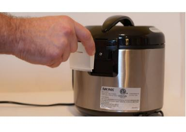
The first step is removing the condensation catcher in order to reach the control panel. We do this by pinching the condensation catcher as shown, on both sides and pull the condensation catcher away from the cooker.
