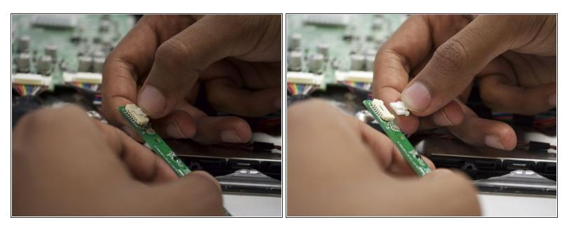
• Remove the light bar by depressing the tab on the white data connector.
