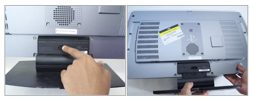
• Remove the base by pushing in the button and sliding out the unit.
