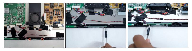
With the Phillips #02 screwdriver, remove the two 5mm length x 5mm head screws located on the left and right side of the light bar board.
